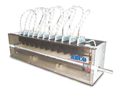
slitter functions that cut dense materials. Shear cut slitters provide clean, precise cuts on flexible materials and provide the longest blade life. Crush cut slitters effectively cut thicker, low density materials such as filter media and nonwovens. These are convenient units for frequent changeovers.
